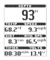
operated from a battery source, the voltage number can be used to determine battery life. The 300TX will operate at voltages from 10 to 20 VDC. Voltages in excess of 20 or less than 10 VDC cause the unit to power off.
